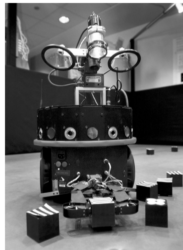
Fig. 1 Darwin VII consists of a mobile base equipped with several sensors and effectors and a neural simulation running on a remote computer workstation. (From [4]).
